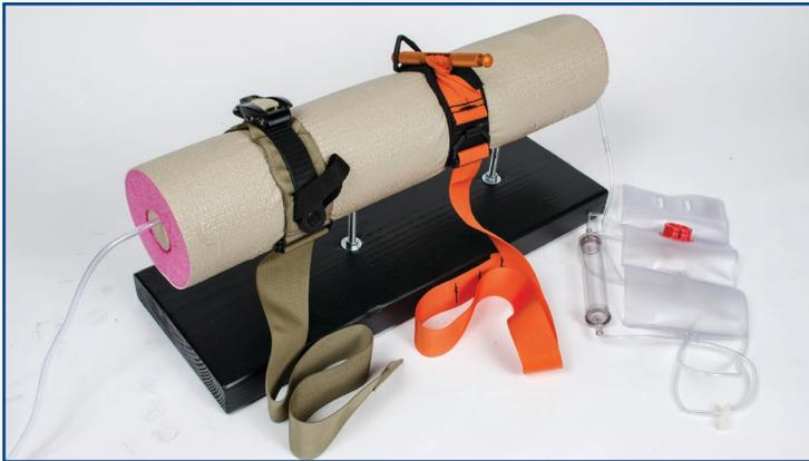
Clamp one end of the tubing and attach a container of colored water to it. An IV administration set works great, or you can improvise something else. Elevate the container above the level of the prop and position the other end to run off into a receiving container. Unclamp the tubing and allow the water to run freely through the prop. This simulates blood flow through a limb. A properly attached tourniquet should stop the flow of water through the tubing.
